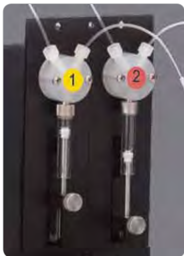
...up to two reagent injectors, programmable with individual injection volumes for each well
