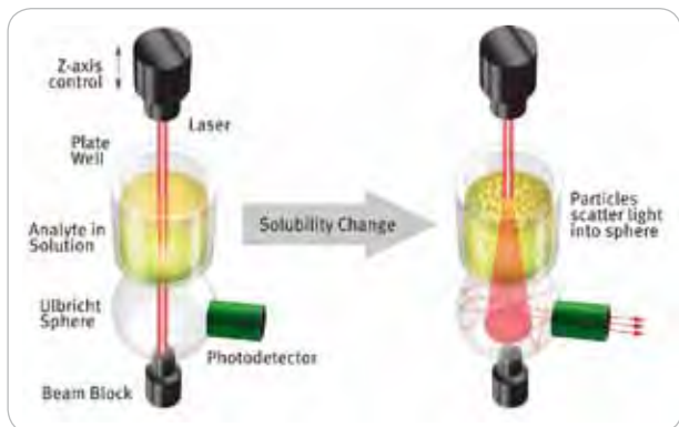
Nephelometry: Scattered light is detected at incident angles of up to 80 degrees, making the NEPHELOstar Plus more sensitive than traditional transmission readers.
