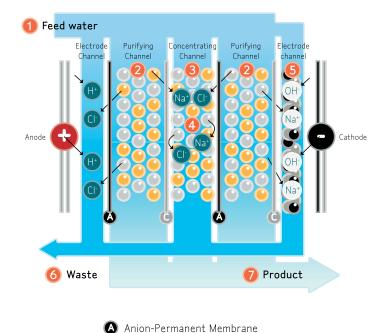
Best-in-class Elix<sup>®</sup> EDI technology The Elix<sup>®</sup> module uses electrodeionization to remove the remaining
