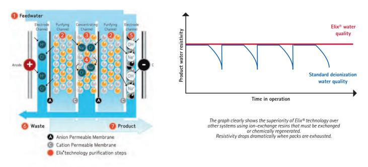
Merck Millipore's Elix<sup>®</sup> module: unique technology based on anion-permeable and cation-permeable membranes; high-quality ion-exchange resin; and activated carbon beads.
