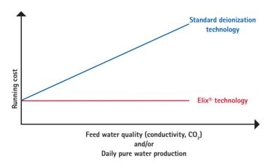
Running costs for a water purification system using Elix® electrodeionization technology or standard ion-exchange resins that must be exchanged or chemically regenerated: With Elix® technology, running costs remain constant, and are independent of feed water quality or pure water use.
