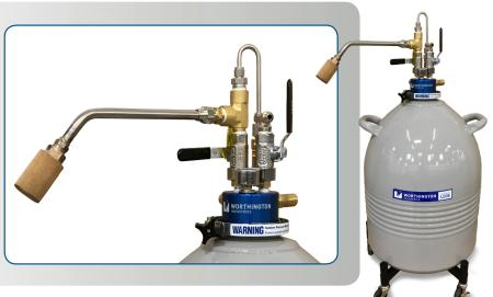
The Liquid Withdrawal Device (LWD) provides convenient pressure transfers of liquid nitrogen from LD25, LD35 and LD50 Dewars. The device clamps directly to the special neck flange that is found under the plastic trim collar around the neck of these containers.
