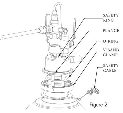
of the hose. If liquid nitrogen is trapped between the valves of the liquid cylinder and the LWD, it has no escape path as it warms and expands. The resulting pressure can cause the hose to rupture and may cause personal injury. The current model LWD is equipped with a pressure relief valve. Previous versions of the LWD must be used with a transfer hose equipped with a pressure relief valve.
