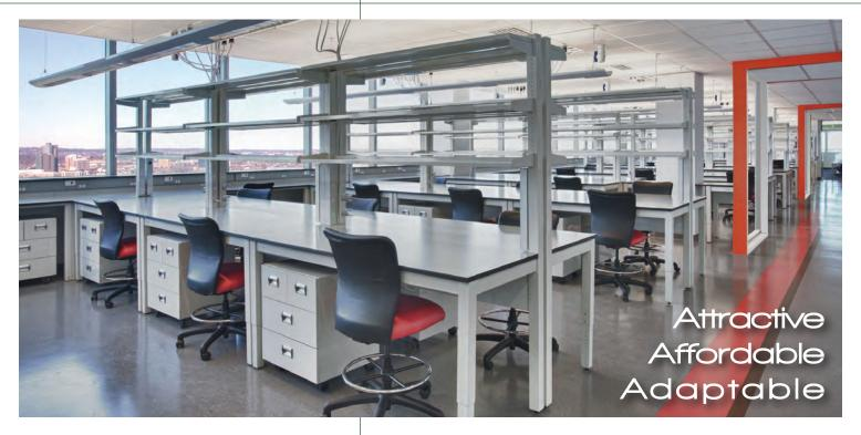
A.T. Villa's Forte system stands uncontested as one of the industry's most cost effective plug and play benching systems. It's unique, telescoping frame allows Forte work surfaces to adjust in 1" increments. Height adjustability is complimented with performance; worktops accommodate uniform loads of 1000lb each and upper shelves accommodate 200lbs each.
