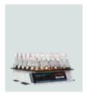
Open-air shakers For shaking in ambient conditions on the bench, in an incubator or in a warm or cold room
