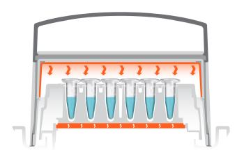
When the ThermoTop is placed on the device, it begins heating immediately. The temperature optimally adapts to the test temperature to ensure that it does not negatively affect the sample. Condensation droplets have no opportunity to form.
