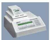
1993 Mastercycler 5330: Eppendorf introduces the first Mastercycler based on peltier technology.
