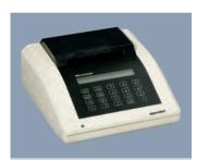
1990 Microcycler: Eppendorf introduces its first thermal cycler using water to heat and cool.
