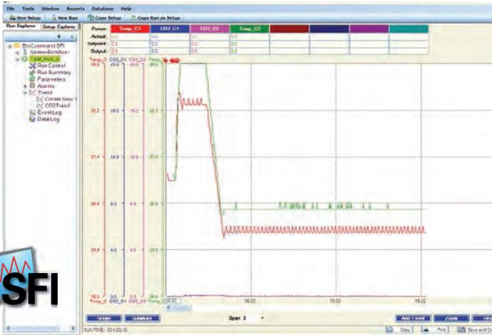
Now you can monitor and permanently record the key operating parameters from multiple shakers, CO<sub>2</sub> incubators, freezers, or other OPC-compliant systems throughout your lab from a single PC.
