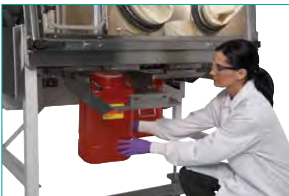
Step 3. Remove container from guides and replace.
