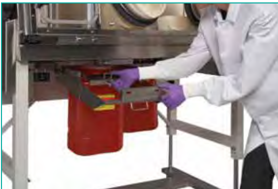
Step 2. Pull down and out container tray. Remove container block.
