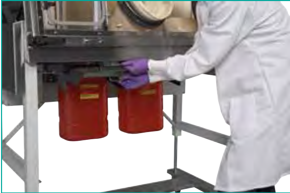
Step 1. Release locking mechanism by pulling handle.
